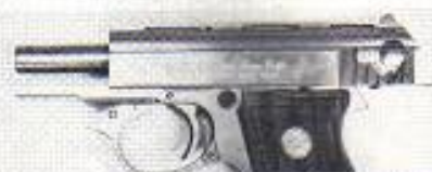
Pulling down Indian's trigger guard allows slide to be drawn rearward and disengaged from frame. Then after being lifted up at the rear, the slide may be moved forward and off frame, exposing barrel and breech and recoil spring.
