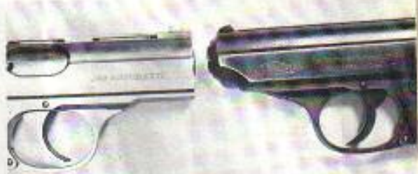
The Indian Arms' .380 is designed after the Walther PPK (right), except for the use of stainless steel and sharply squared muzzle.
