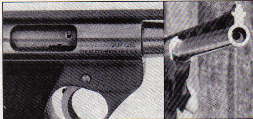
Because the Baby is not a production item, it wears a serial number indicating its experimental status. The deep recessed crown of the muzzle is intended to give the .22 that intimidating big-bore look.
